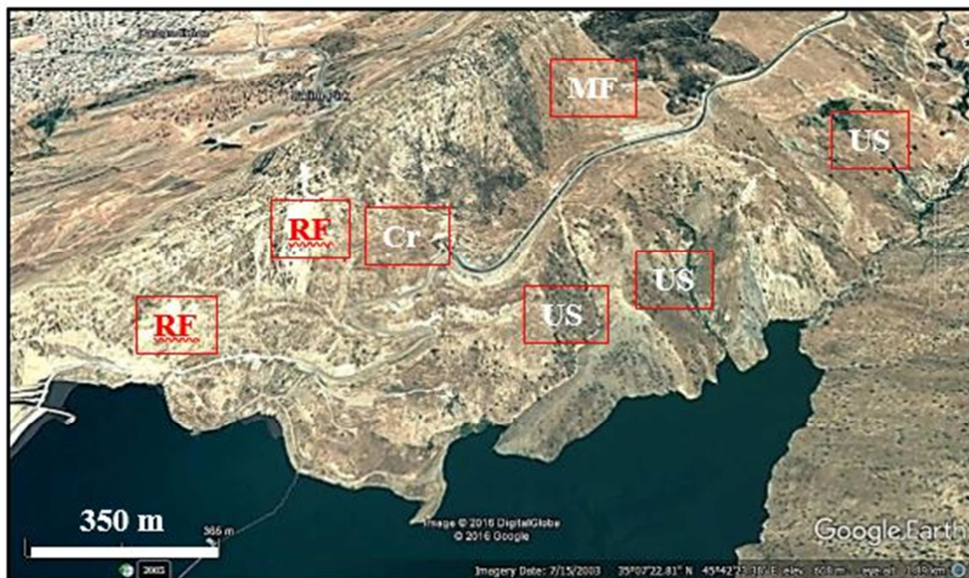
Figure 3: Google Earth image showing erosional slopes. Note the majority of the slopes are unstable (US), also note rock fall (RF), Mud Flow (MF), Landslide (LS) and Creep (Cr) phenomena.
